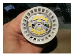
In order to find the voltage and current used by the LED array I remounted the LED array to the heat sink and connected a dc voltmeter and ammeter to the circuit. Although the array seems to be electrically isolated from the line, to be on the safe side, I fed the bulb through an isolation transformer and used a Variac to adjust the input voltage from 0 to 125Vac.
