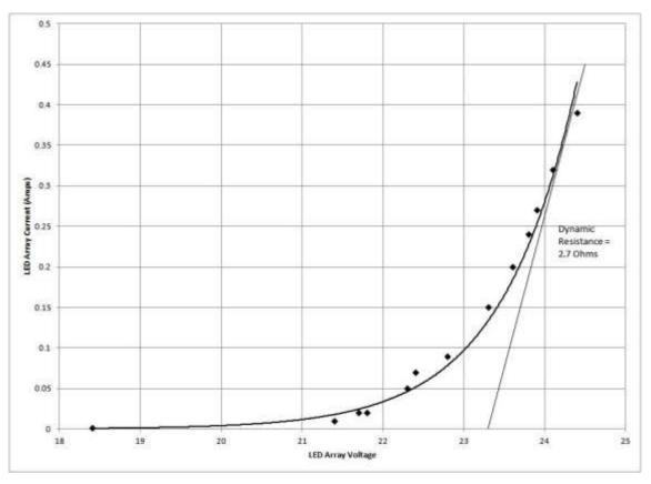
Figure 3 LED Array V-I Curve
