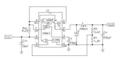
Reconfiguring the board from buck mode to boost mode took some careful work with a motor tool and some creative relocation of the inductor and Schottky diode. I changed the timing capacitor and R2. We really don't care about output voltage ripple because the human eye cannot see the 100kHz flicker of the LED but I put a 22µF
