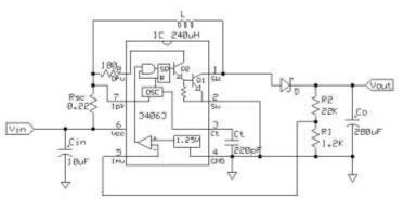
EMCOMM or portable operation. The efficiency is nearly Figure 5 DSU Reconfigured as Boost Mode
